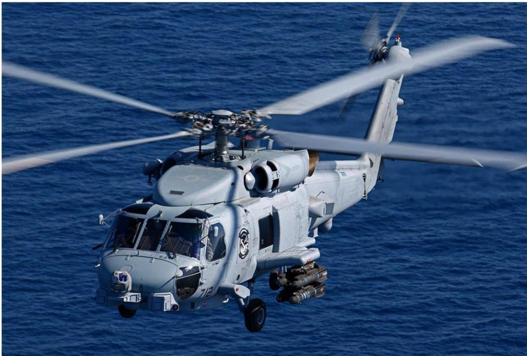
Figure 4.5. SH-60R, utilizing an articulated rotor system. Photo courtesy of LockheedMartin.com
