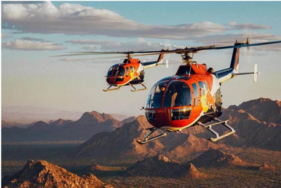
Figure 4.3. A Bo105 which utilizes a hingeless rotor system, photo courtesy of RedBull.com
