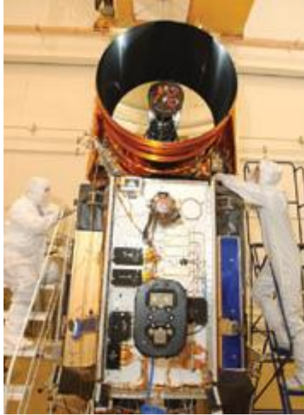
Figure 1-8 - GLAS LIDAR system [17]
