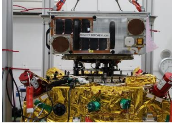
Figure 3-1 - ELSA-D Magnetic Dock Capture System [21]
