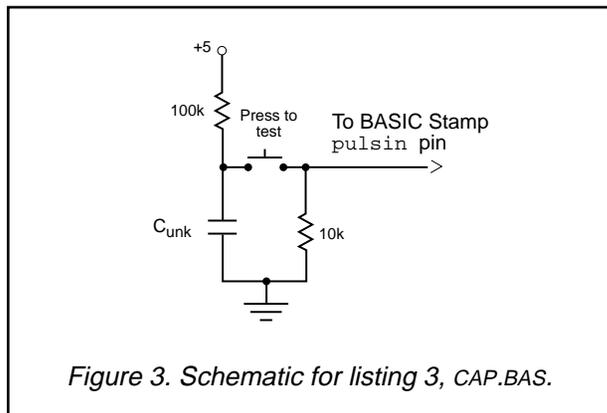
be sure that the charging resistor (100k in this case) is about 10 times the value of the discharge resistor. This ensures that the voltage at the junction of the two resistors when the switch is held down is a definite low (0) input to the Stamp.
