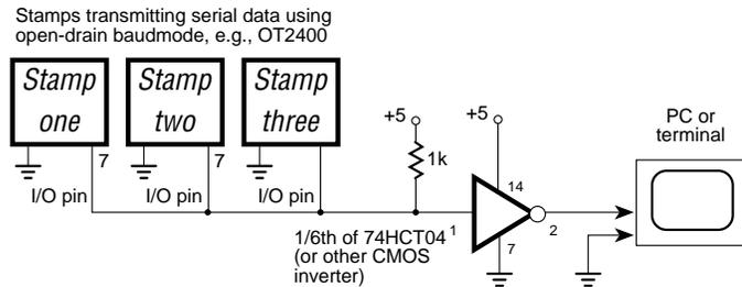
To understand why you must use the “open” serial modes on a network, consider what would happen if you didn’t. When none of the Stamps are transmitting, all of their Serout pins are output-high. Since all are at +5 volts, no current flows between the pins. Then a Stamp transmits, and switches to output-low. With the other Stamps’ pins output-high, there’s a direct short from +5 volts to ground. Current flows between the pins, possibly damaging them.
