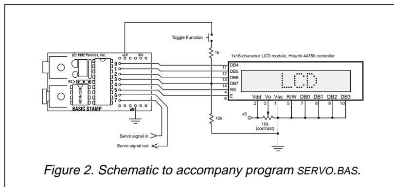
Figure 2. Schematic to accompany program SERVO.BAS.
