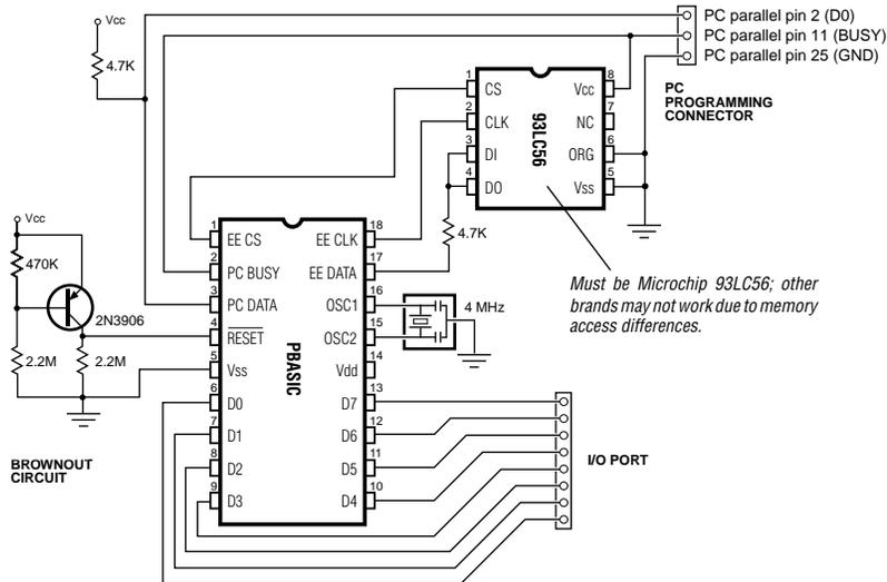
\* The BS1-IC has a slightly different schematic (it uses a different reset circuit, and it includes a 5-volt regulator). However, this schematic serves as an example of how simple the BASIC Stamp circuit is to implement.
