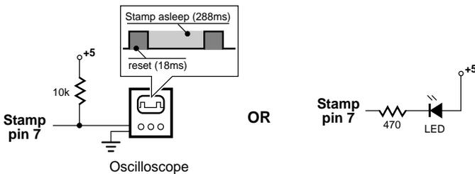
Use either of these circuits to observe the output glitch when the Stamp awakens from a Nap. Pin 7 is output low while the Stamp is asleep. When it resets, all pins switch to input, allowing the resistor to pull pin 7 high (left) or causing the LED to blink off (right).
