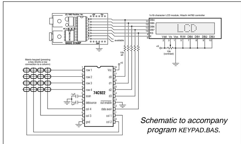
outputs a “data available” bit and 4 output bits representing the number of the key pressed from 0 to 15. A companion device, the 74C923, has the same features, but reads a 20-key pad and outputs 5 data bits.
