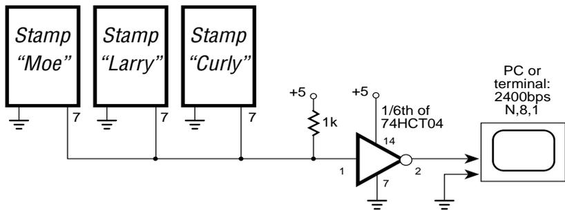
Figure 4. Serial network of Stamps using open-drain output.
