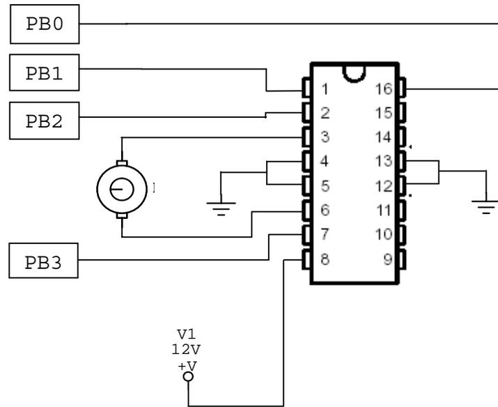
Figure 17: The printer carriage motor circuit using the H-bridge
