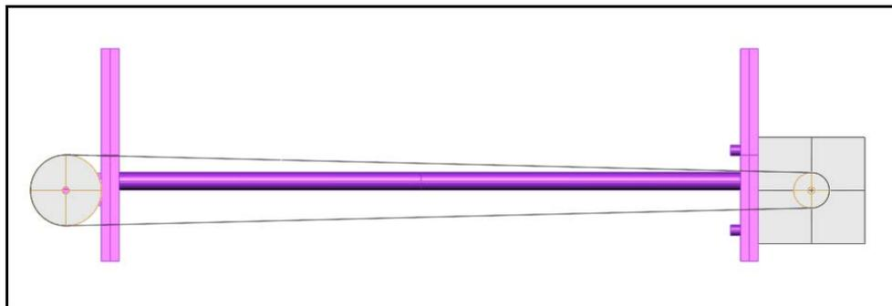
*Figure 7: Front view of the printer carriage mechanism, showing the belt and pulleys*
