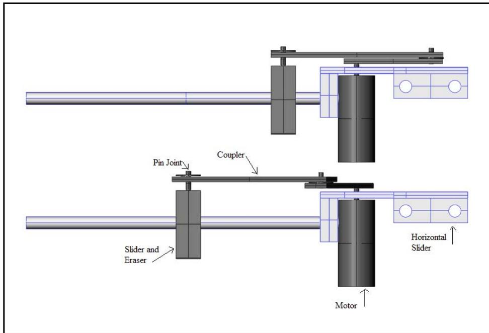
*Figure 4: Side view of the four-bar slider-crank mechanism at two different positions*
