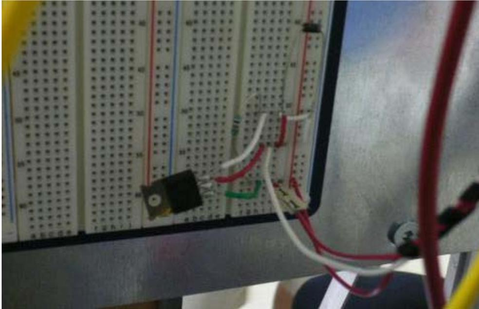
*Figure 16: Photograph of the DC motor driver circuit*
