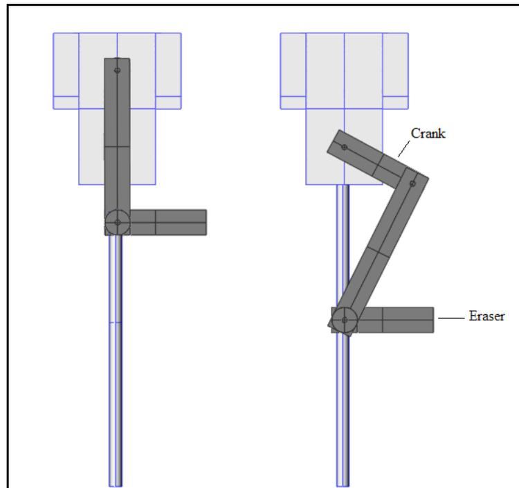
*Figure 3: Front view of the four-bar slider-crank mechanism. The drawing on the left represents the four-bar in its initial position, and the figure on the right illustrates the four-bar as the slider moves along the vertical rod.*
