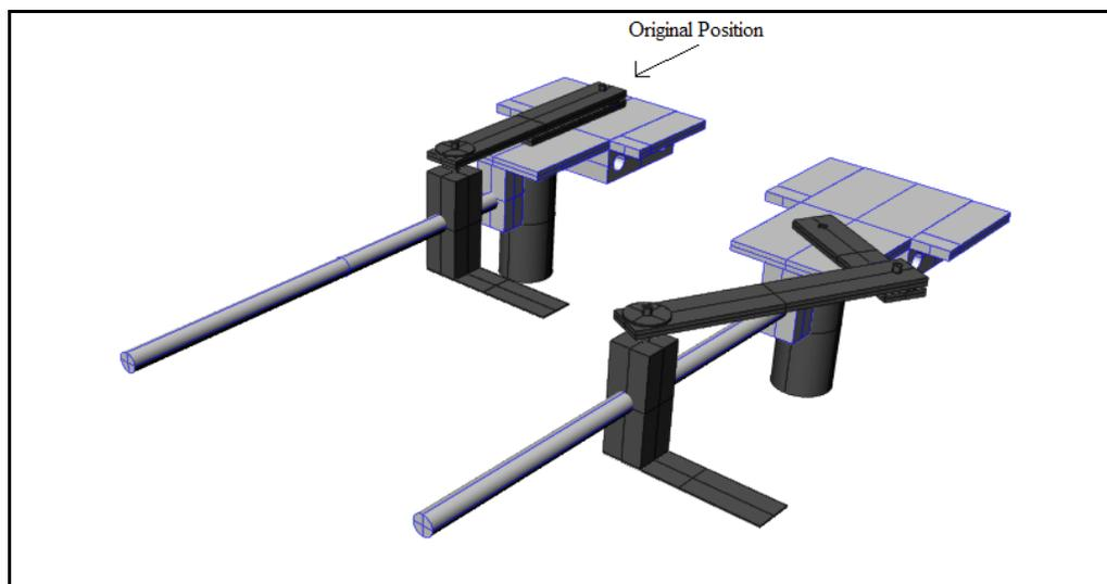
*Figure 5: Perspective view of the four-bar slider-crank mechanism at two different positions*
