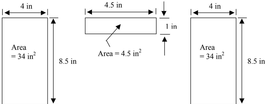
*Figure 4: Areas of the prototype board to be erased*
