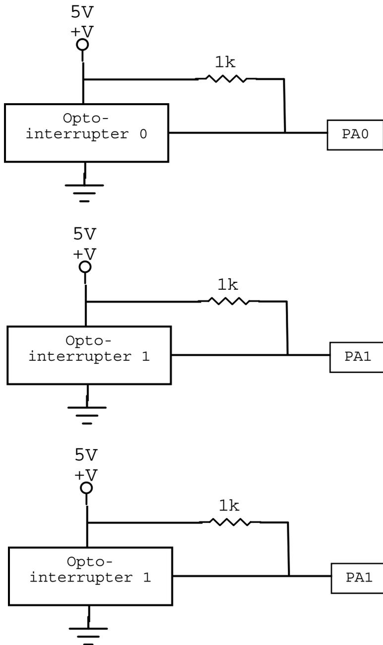
Figure 19: Opto-interrupter switch circuits.
