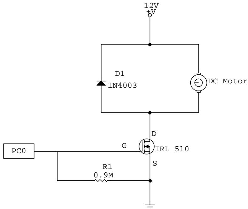
*Figure 15: DC Motor Driver Circuit. The circuit uses an IRL 510 power MOSFET*
