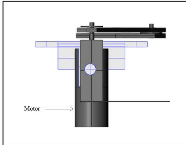
*Figure 8: DC motor which for the crank on the four-bar mechanism*
