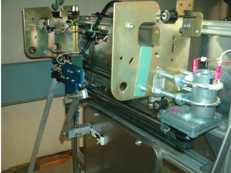
*Figure 10: Photograph showing the placement of the printer carriage DC motor in relation to the rest of the prototype*
