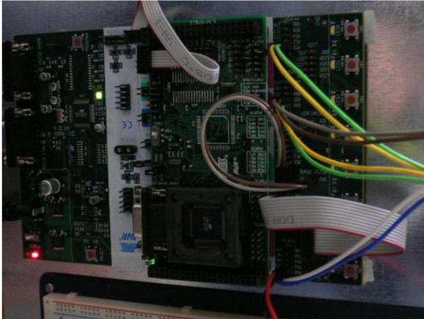
*Figure 14: The Atmega Atmel 128 microcontroller*
