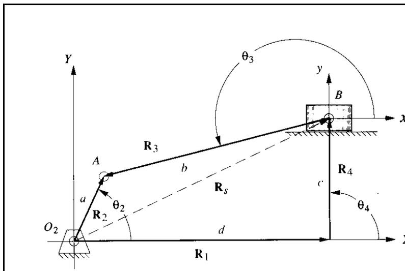
Figure 24: Diagram of the four-bar slider-block mechanism
