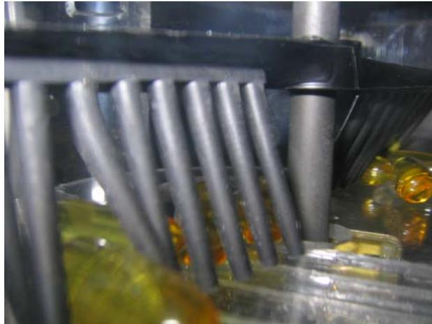
**Figure 8: Picture of the brush strip that was cut and then glued using epoxy to the airplane propeller.**
