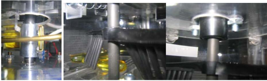
**Figure 3:** Pictures showing the connection of the Dc motor to the shaft through the coupling and to the aluminum stock through to the mounted bearing at the top of the pill dispenser.
