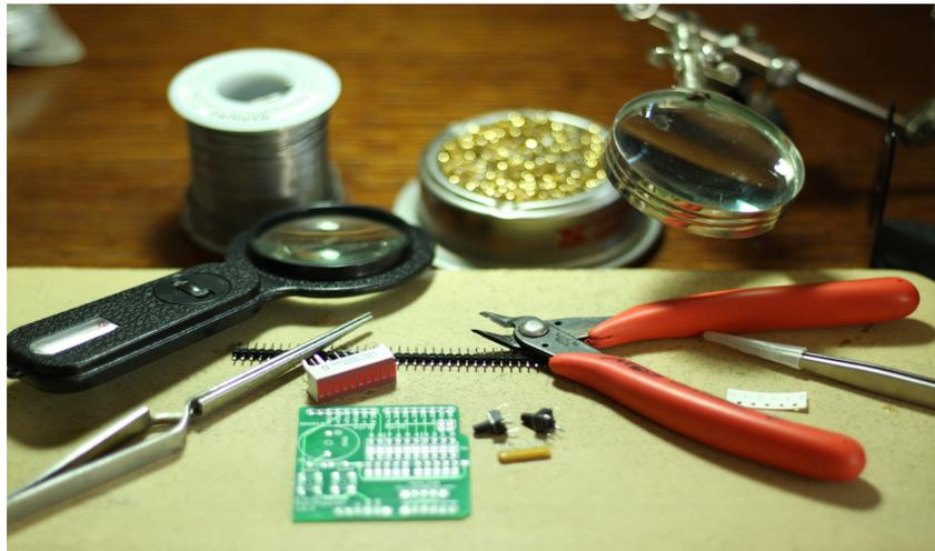
*Illustration 1: Parts and tools ready for hot soldering action*
