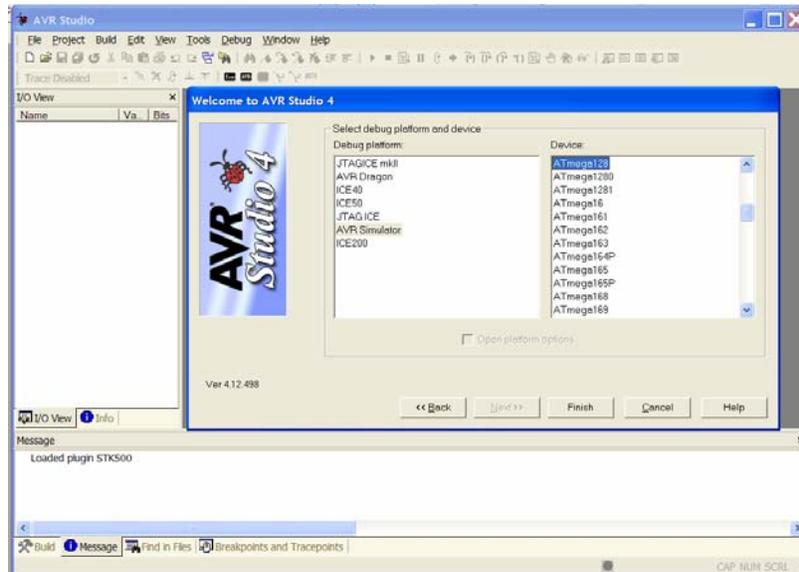
**Figure 3.** AVR Studio Project Wizard Debug Platform and Device Screen.
