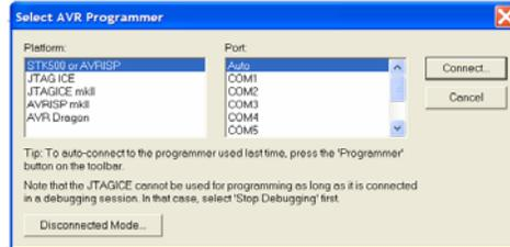
**Figure 4.** Select AVR Programmer dialog box. This window allows you to choose the platform and COM port with which to program the ATmega 128. The selection on the left side should be STK500 or AVRISP and that on the right should be Auto (to auto-detect for an available COM port on your PC).
