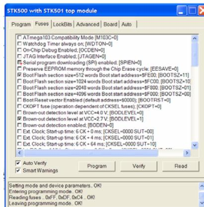
**Figure 5.** Fuse dialog box. This window allows you to select the fuses on the ATmega 128.
