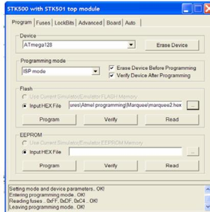
**Figure 6.** Program dialog box. This window allows you to navigate to the hex file to be downloaded to the microcontroller.
