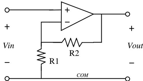
**Figure 3** A non-inverting amplifier. The gain of the amplifier is  $(R_1+R_2)/R_1$ .
