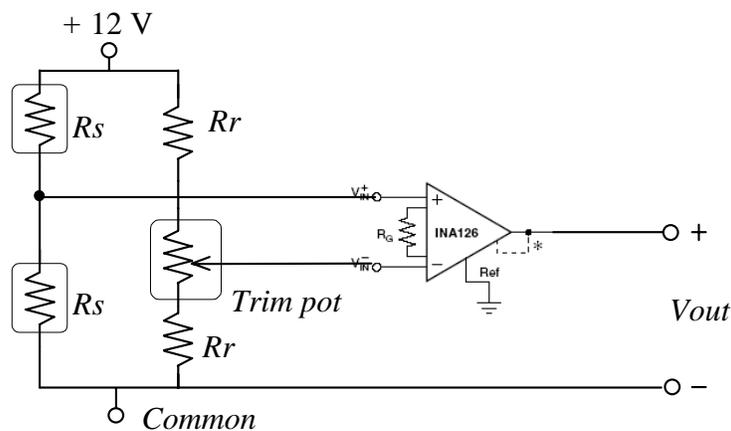
**Figure 6** The electronic scale circuit schematic. The strain gauges are placed in a Wheatstone bridge, and an instrumentation amplifier amplifies the bridge voltage. Although not shown, the supply voltages for the INA126 are ±12 V.
