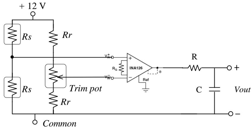
**Figure 6 The electronic scale circuit with low-pass filter.** The low-pass filter will attenuate high frequency noise.
