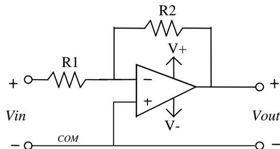
**Figure 2** An inverting amplifier. The gain of the amplifier is  $-R2/R1$ . It is always a good idea to keep the leads to the inputs of the op-amp and the feedback loop short to minimize noise pickup.
