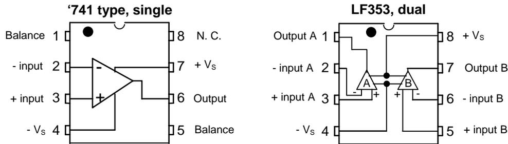
**Figure 1** Examples of single and dual op-amp IC packages. The ‘741 was one of the earlier, but still very common, general purpose IC op-amps. Both the ‘741 and LF353 should be powered with symmetrical positive and negative power supplies (see their data sheets for maximum limits). We will use the LF353 dual op-amp in this experiment.
