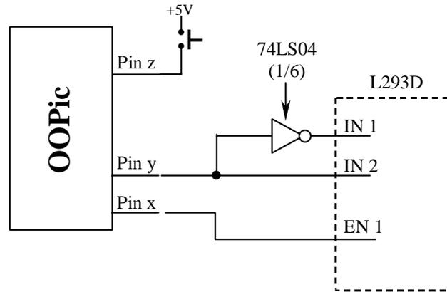
**Figure 4.** Connections to the OOPic, the 74LS04, and the L293D. Note that the connections for  $V_S$  and +5 are not shown on the L293D, but need to be connected.
