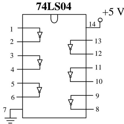
**Figure 2.** 74LS04 connections. The 74LS04 is a logic IC containing six inverters, also called NOT gates. The schematic symbol for a NOT gate is a triangle with an open circle at the end.
