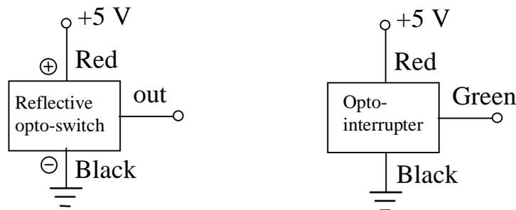
**Figure 1.** Opto-switch connections for photoreflexive and photointerrupter switches
