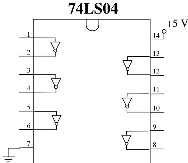
**Figure 2.** 74LS04 connections. The 74LS04 is a logic IC containing six inverters, also called NOT gates. The schematic symbol for a NOT gate is a triangle with an open circle at the end.
