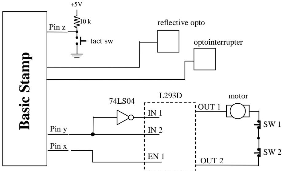
**Figure 5.** Printer Carriage Motion Controller. The carriage is driven between limits set by the two opto-switches continuously after the program detects that the tact switch has closed.
