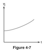
Both thixotropy and rheopexy may occur in combination with any of the previously discussed flow behaviors, or only at certain shear rates. The time element is extremely variable; under conditions of constant shear, some fluids will reach their final viscosity value in a few seconds, while others may take up to several days.
