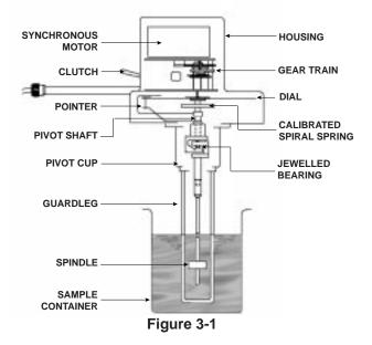
Below the main case is the pivot cup through which the lower end of the pivot shaft protrudes. A jewel bearing inside the pivot cup rotates with the dial or transducer; the pivot shaft is supported on this bearing by the pivot point. The lower end of the pivot shaft comprises the spindle coupling to which the Viscometer's spindles are attached.
