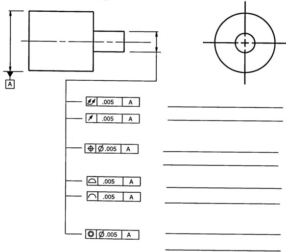
7. Only one of the controls above are allowed to have the material condition modifiers MMC or LMC applied to the feature tolerance. Which one is it?
