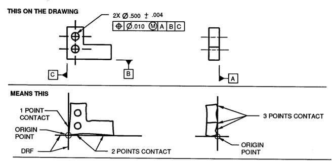
In the figure above, an imperfect part is shown loaded on the datum reference frame according to the order designated in the feature control frame. In the following examples, sketch an imperfect part loaded on the datum reference frame according to the applicable feature control frame. Also, specify the points of contact on each plane and identify the origin point.
