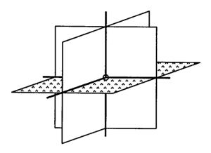
2. The datum reference frame is three mutually perpendicular planes. In engineering, it represents the surface of a drafting table, the straight edge and the 90 degree triangle or the coordinate system in CAD. What equipment does it represent in manufacturing?
