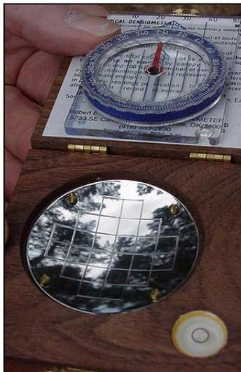
**Figure 19: Spherical Densitometer**
