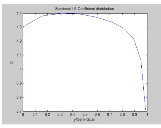
Figure 7.5 – 5 degrees angle of attack lift distribution
