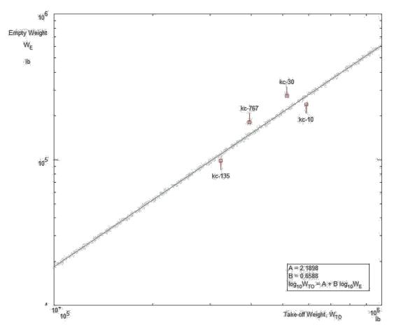
Figure 4.1 – Empty weight vs. takeoff weight relationship for tankers
