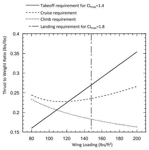
Figure 5. 7 – Manual performance requirement results
