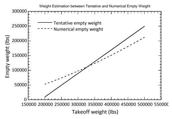
Figure 4.3 – Weight estimation between tentative and numerical empty weight
