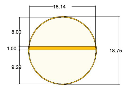
Figure 6. 3 – Cabin cross section
