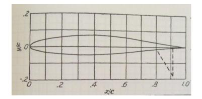
Figure 7. 2 – NACA 641-212 airfoil
