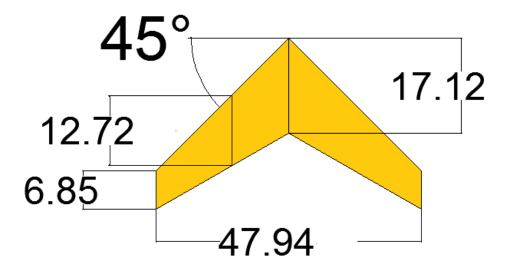
Figure 8. 2 – CAD model for the horizontal stabilizer
