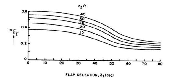
Figure 7.8 – Section lift effectiveness parameter for fowler flap
