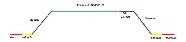
Figure 2. 4 – Mission profiles for cargo transfer mission and medical evacuation mission
