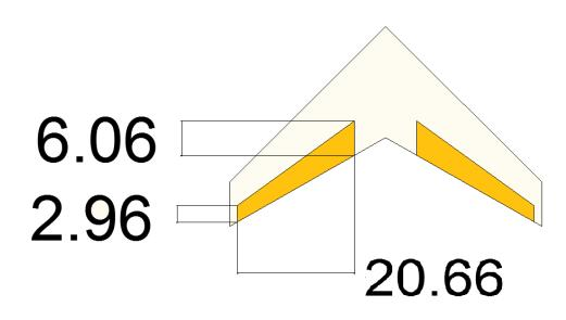
Figure8. 4 – CAD model of elevator
