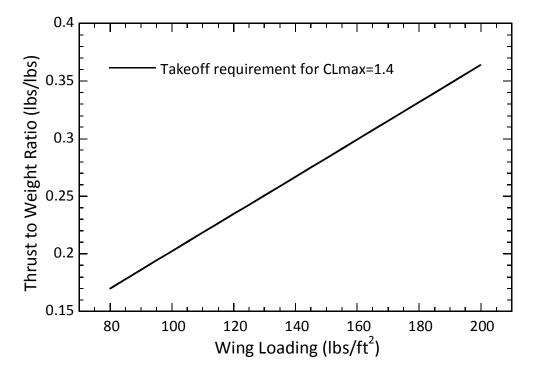
Figure 5. 3 – Takeoff distance requirement for CLmax=1.4
