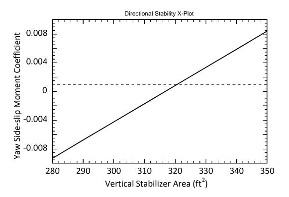
Figure11.2 – Directional stability X-Plot
