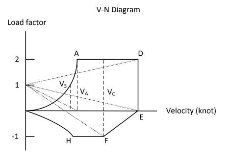
Figure13. 1 – V-N diagram for the KC-X
