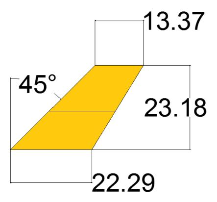
Figure 8. 3 – CAD model for the vertical stabilizer
