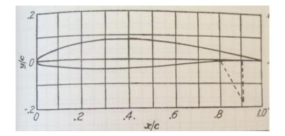
Figure 7. 3 – NACA 641-412 airfoil
