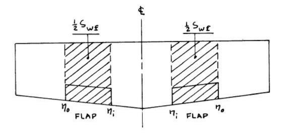
Figure 7. 7 – Definition of flapped wing area
