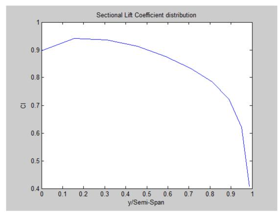
Figure 7. 4 – Zero angle of attack lift distribution
