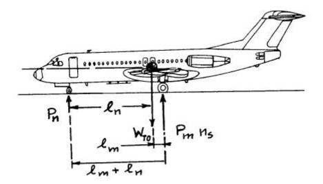
Figure 10. 1 – Static load geometric for tricycle gears
