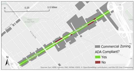
Figure 20: ADA sidewalk Compliance on Alum Rock Avenue
